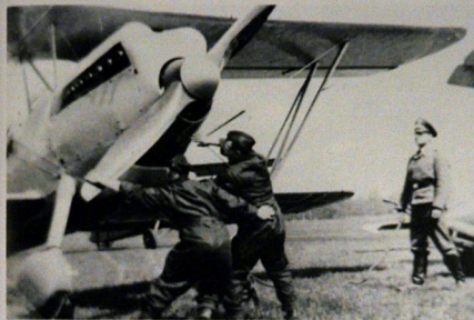
LEFT: Contact Two mechanics swing the propeller of this Ar 68 F in order to start its BMW V1 engine. It would appear that the cowling for the cooling system is open in this photo.
