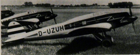
ABOVE: One of the most beautiful aircraft of the between war period, the He 70 was designed by the Günter brothers as a fast transport. The first passenger carrying He 70s were used by Deutsche Lufthansa on its Berlin-Hamburg-Köln-Frankfurt am Main service, and later other routes inside Germany. With the birth of the Luftwaffe, two military versions were produced, the He 70 E and F, these being tested as fighter, reconnaissance and bombing aircraft.
