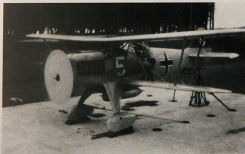
ABOVE: The Ar 68 F could easily be distinguished from its Jumo powered counterpart by its much more bulky engine installation. The variant was delivered to the Luftwaffe from the summer of 1936, first to I/JG 134 at Dortmund and later to I/JG 131 at Jesau. It had been hoped that the Ar 68 would supersede the He 51 but trials conducted between the two aircraft by Ernst Udet proved that the former did not have much of an improved performance, but was easier to maintain.
