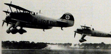
ABOVE: Three of the nine pre-production batch He 51A-0 series aircraft taking off. The nearest machine D-IQEE, also shown middle right, shows the standard port side tail markings of the time, a red band with the Hakenkreuz inside a white circle. All the pre-production machines were finished in silver coloured aluminium dope.
