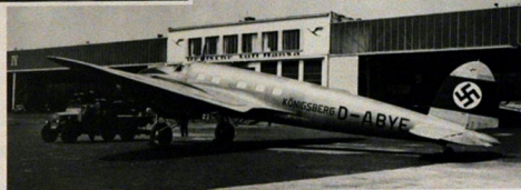
ABOVE AND RIGHT: Two views of He 111 C04, D-ABYE 'Königsberg' which was delivered to Luftwaffe in the summer of 1936. The aircraft could carry ten passengers at a maximum speed of 315 km/h (196 mph) but was considered by the airline to be too expensive for commercial operation. Nevertheless by the summer of 1937 the type was operating on no fewer than 16 routes.
