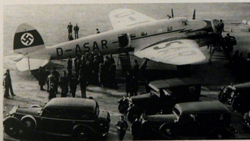
LEFT: The He 111 V16, D-ASAR, had straight wings similar to those later fitted to the He 111 bomber widely used by the Luftwaffe. The aircraft was used by Erhard Milch as his personal transport.
