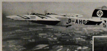
ABOVE: Early trials with the Do 11 were to show that the flying characteristics of the aircraft were far from perfect. Under certain conditions the wings vibrated alarmingly, necessitating the redesign of both the wing and enlargement of the vertical tail surfaces. The resulting variant, the Do 11 D seen here, was better, although problems with the retractable undercarriage were such that the unit was locked down on all service aircraft.
