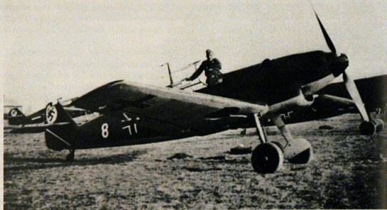
ABOVE: A line-up of factory fresh Bf 109 Bs after delivery to II./JG 132. The superb Messerschmitt fighter began to replace the He 51 and Ar 68 in Luftwaffe service from the spring of 1937. Its introduction brought a change to Jagdwaffe camouflage, all Bf 109s of the period having black-green (RLM colour 70) and dark green (71) uppersurfaces with pale blue (65) undersurfaces.
