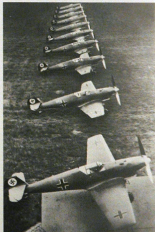
BELOW: When the first 25 Bf 109 B-1s were delivered to II./JG 132 'Richtsholen' in February 1937, they were fitted with the large wooden fixed two-bladed propeller and were camouflaged in black-green and dark green. They were however to retain the early style Balkenkreuz national insignia with thin white outlines and black edging. They also carried the original black Hakenkreuz on a white circle painted over a red tail band.
