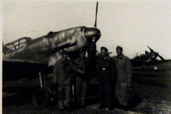
LEFT: Some of the last production Bf 109 Ds were delivered to the Luftwaffe in the later style fighter camouflage with pale blue fuselage sides. These aircraft, from an unknown unit, but probably a training school, have their upper surfaces painted in either two greys (RLM colours 74 and 75) or perhaps in a mixture of dark green (71) and RLM grey (02). Many early C and D variants were ultimately transferred to training schools.
