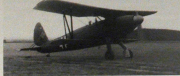
ABOVE: It was by no means unusual for the wheel spats of the Ar 68 to be removed to ease maintenance. This aircraft has black-green and dark green undersurfaces. Many early machines continued to see service but were gradually transferred to training schools.
