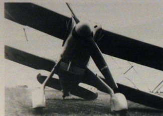
ABOVE: The port undercarriage leg of this He 51 collapsed on landing at Jever airfield. The aircraft, which was operated by 1./KüJ.Gr 136, carries its five character code 60+41 painted in black on both sides of the fuselage, on top of the upper wing and beneath the lower wing.
