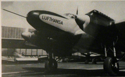
ABOVE AND RIGHT: Two views of He 111 C04, D-ABYE 'Königsberg' which was delivered to Luftwaffe in the summer of 1936. The aircraft could carry ten passengers at a maximum speed of 315 km/h (196 mph) but was considered by the airline to be too expensive for commercial operation. Nevertheless by the summer of 1937 the type was operating on no fewer than 16 routes.
